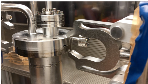
Figure 4: Clamp Openers applying Model 1 Clamps.
